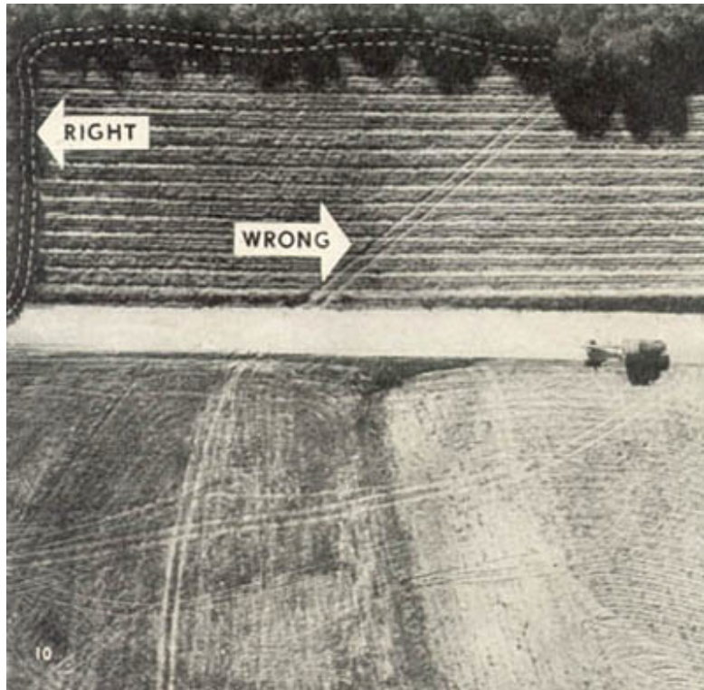
FIGURE 4. Tracks crossing natural terrain lines are noticeable, while tracks parallel to natural terrain lines are likely to be overlooked.
